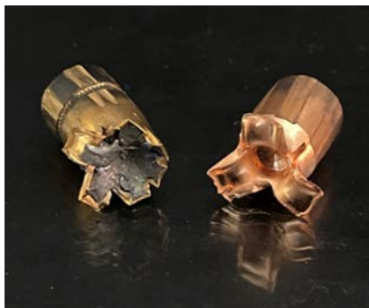
Jeans into gel test HST 124 grain vs VX9 96 Grain Left bullet HST Right Bullet VX9
